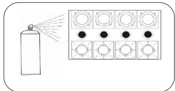
4. Fold the cardboard template into a box. Spray paint the sensors and the adapters and let dry thoroughly before assembling.
