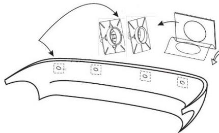
4. Peel off the remaining adhesive liner and align the adapters on the 4 holes previously drilled in the bumper.
