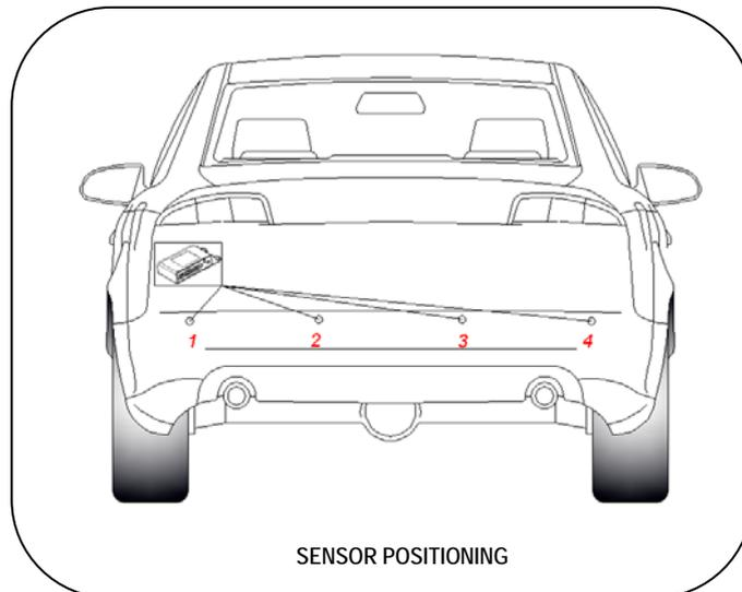
7. Space out the supplied adhesive cable clips along the bumper, insert the cable ties and secure the wires in place. Bundle up any excess cables.
