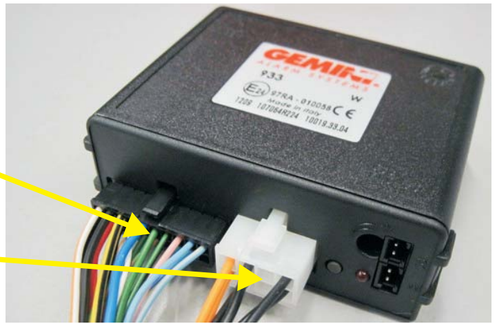
Plug the wiring connectors into the corresponding outlets on the alarm unit.
